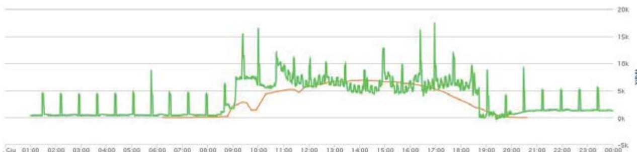
Fig. 5 –Power profile at the interface with the grid (green) and power generated by the PV plant (red)
