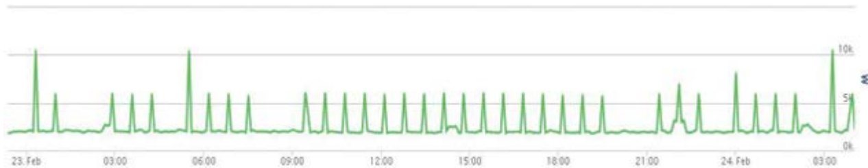
Fig. 4 – MAVEL's power load, non-working day
