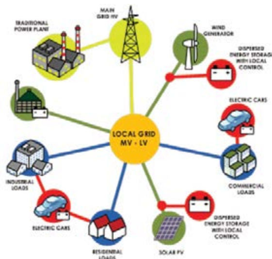
Fig. 7 Configuration of the electrical system in the future scenario with dispersed energy storage with local control and electric cars
