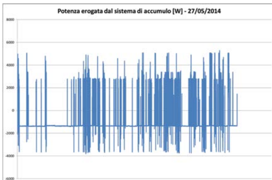
Fig. 14 Power flows of the ESS apparatus in the experimental test in TecnoCity ([W] vs time, one day time window)
