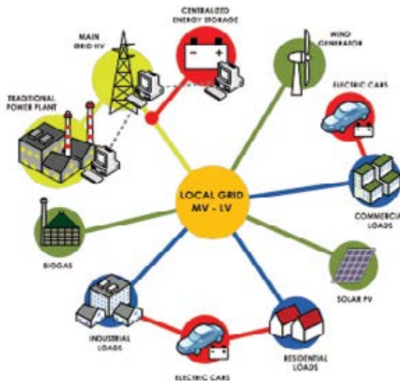
Fig. 6 Configuration of the electrical system in the future scenario with centralized energy storage and electric cars
