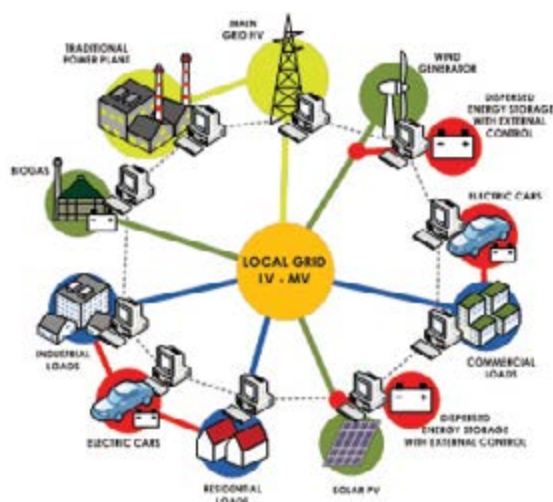
Fig. 8 Configuration of the electrical system in the future scenario with dispersed energy storage with external control and electric cars
