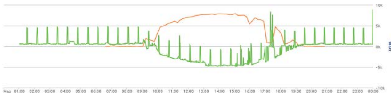
Fig. 6 – PV power generation (red line) and grid interface power (green line) of a non-working day with good solar radiation
