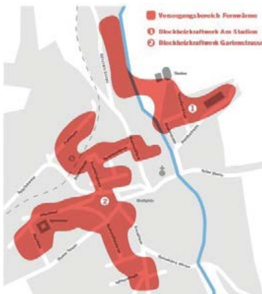
Figure 5: Schematic view of the two district heating grids in Grafing (left) and detailed view of the district heating grid “Gartenstraße” (right) [Rothmoser]
