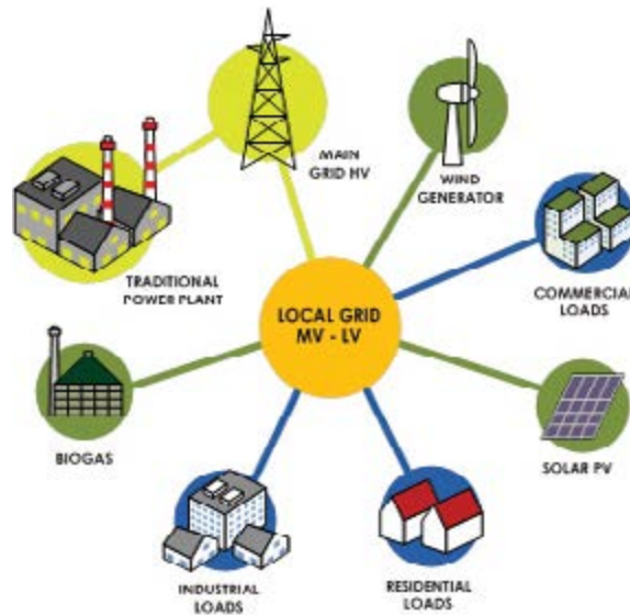
Fig. 5 Configuration of the local electrical system in the current scenario
