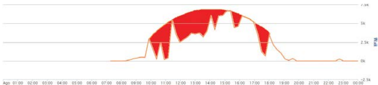
Fig. 8 – PV energy stored in the battery (red area)
