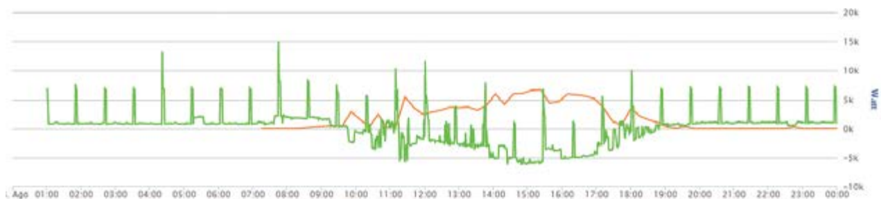
Fig. 7 – Power profile of the Smart Node in configuration Load-RES-Storage-Grid
