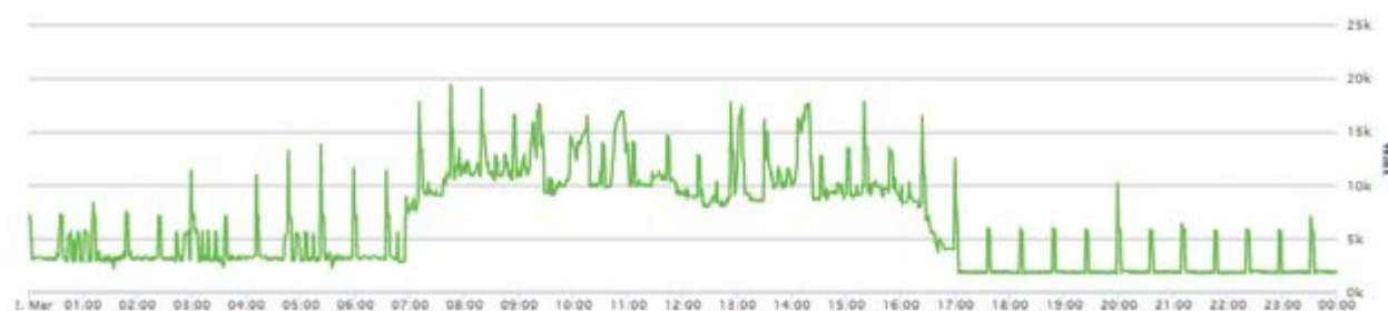
Fig. 3 – MAVEL's power load, working day
